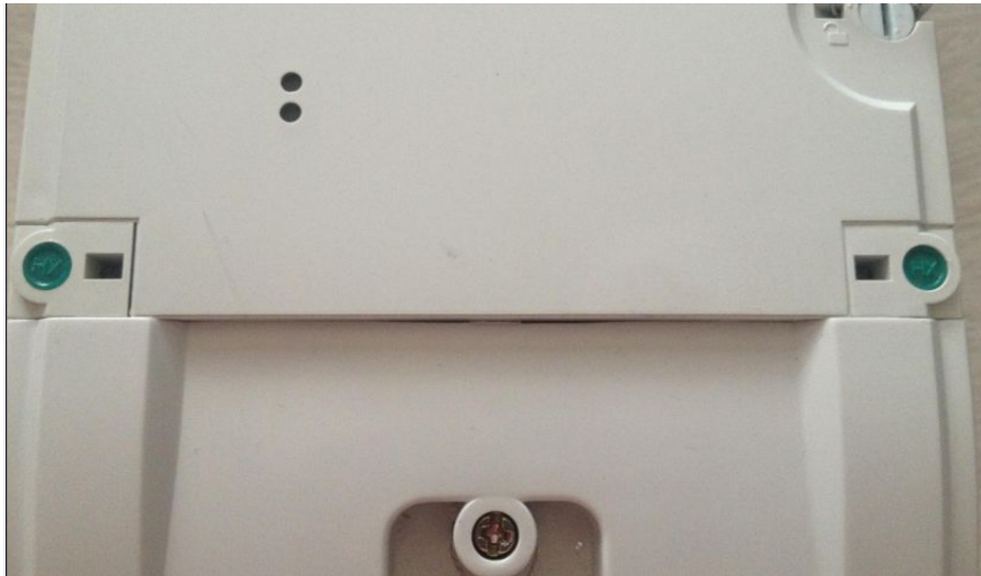
Figure.3.2.2 meter cover seal
