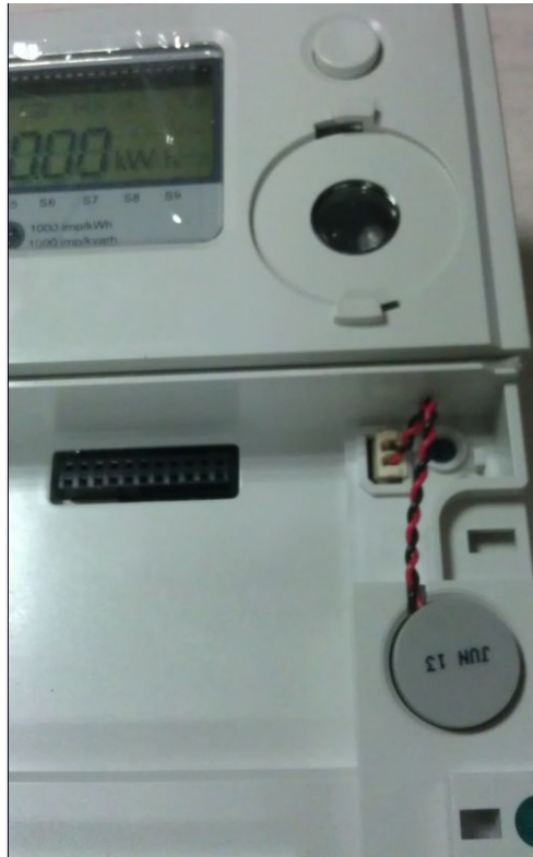
Figure 4.17.4.4 Battery installation view
